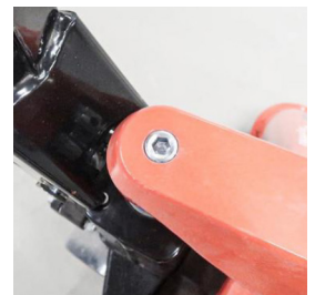
The fork height is adjustable to save pump strokes.
