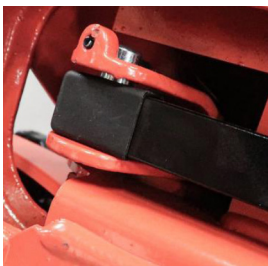
Movable parts with tight tolerances without metallic contact
